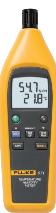
Quickly take accurate humidity and temperature readings in the air. Temperature and humidity are two important factors in maintaining optimal comfort levels and good indoor air quality. The Fluke 971 is invaluable for facility maintenance and utility technicians, HVAC-service contractors, and specialists who assess indoor air quality (IAQ). Lightweight, rugged, and easy to hold, the Fluke 971 is the perfect tool for monitoring problem areas.
